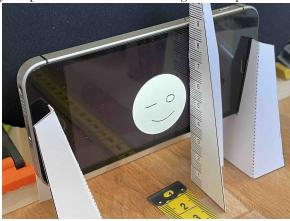
Find a surface that is at least 140cm long where you can set things up as shown to the right. First tape the tape measure to the surface so that it does not move.
