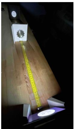
Place the lens at x=40cm. Notice that a small notch has been cut out of the bottom edge of the lens holder so that it straddles the tape measure without touching it.
