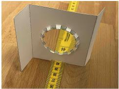
Place the observation screen at  $x=80\mathrm{cm}$ . There is a notch in the observation screen too. Move the screen around until you find the location where the image is as sharp as possible. Record the location  $x_{\mathrm{lens}}$  of the lens and the location  $x_{\mathrm{image}}$  of the image .
