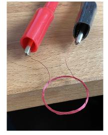
When the coil is connected DMM leads as shown, use the DMM to measure the resistance. If the resistance is greater than  $2\Omega$  then the ends need to be burned and cleaned again.
