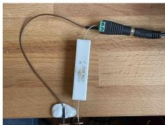
The resistor lead can be shaped a bit with the pliers to make a cradle for the ends of the loop so that the loop does not fall off so easily.
