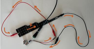
The DMM can measure the amount of the current, if you force the current to pass through the meter as shown below. Notice the connection of the leads to the DMM and the position of the dial are not the same as when you measure voltage. Write down the current you measure, be sure to note the units.
