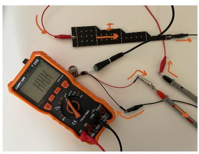
Now connect the DMM to the circuit as shown below, and measure the current again. Write down the value of the current.
